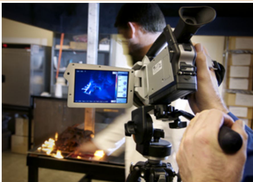
A new thermal imaging camera gathers precise temperature information, providing fire scientists a more detailed understanding of fire behavior.
