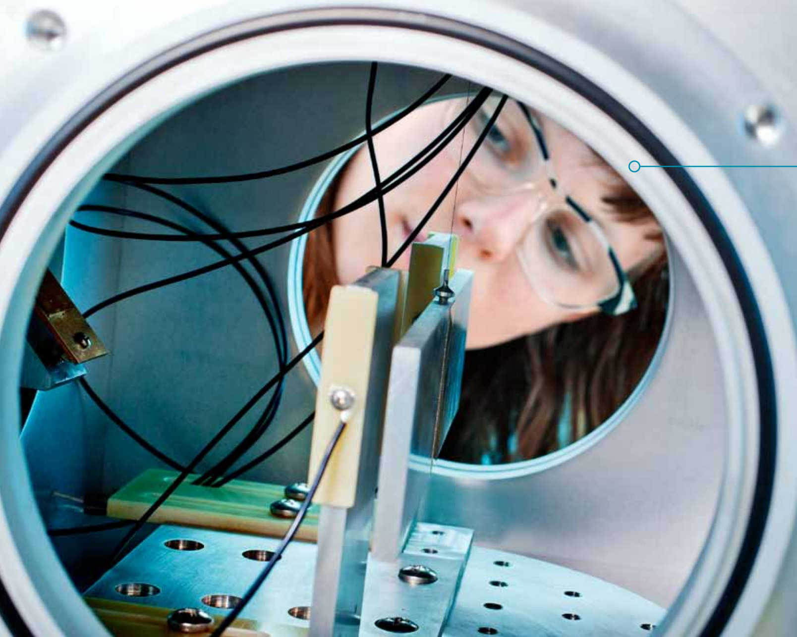
Student Holly Leopardi uses the Department of Physics & Astronomy’s torsion pendulum, which is used to measure gravity at infinitesimal distances.
