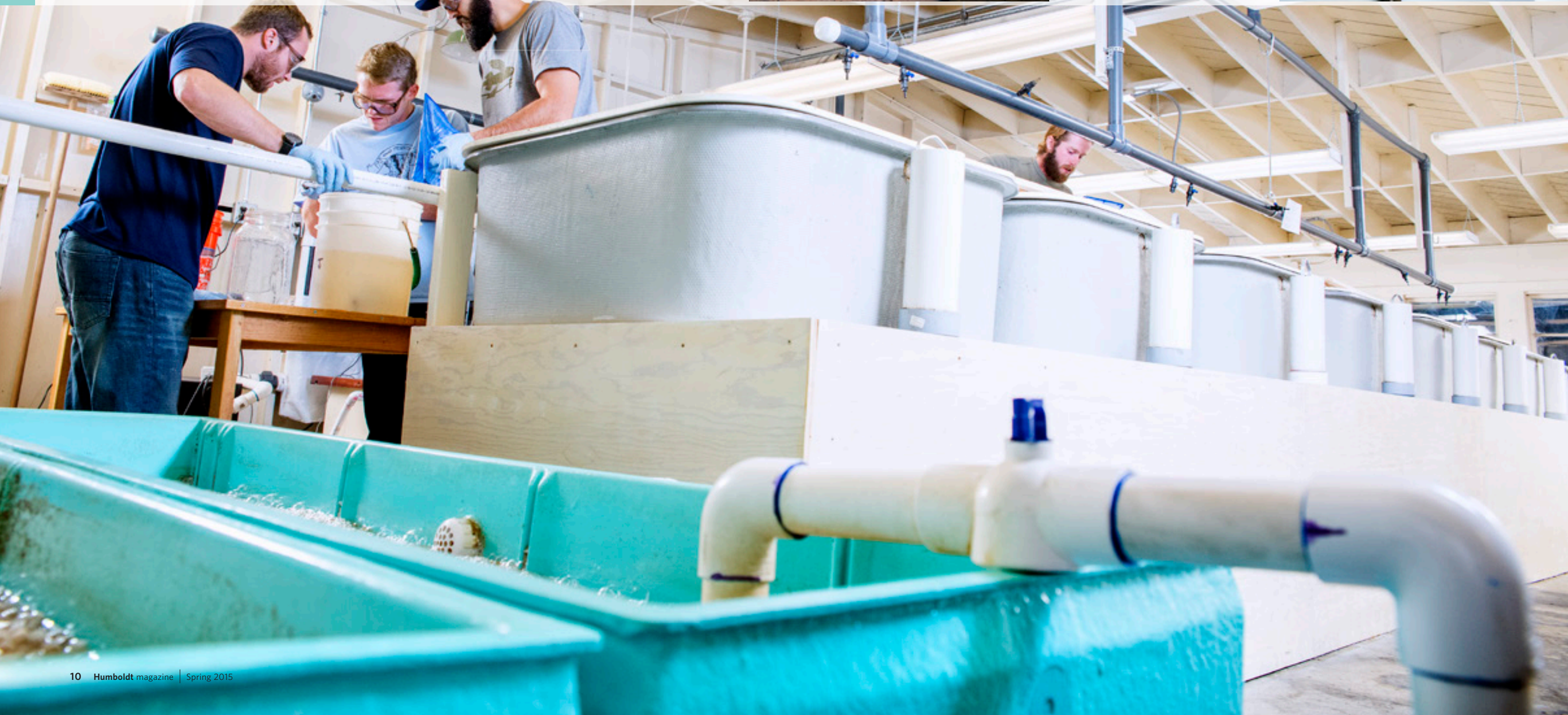
LEFT: These plastic biofilter media remove ammonia from the water, which is toxic to fish. ABOVE: A student measures the length and weight of a juvenile trout. RIGHT: Students monitor the fish's health and maintain a delicate balance of bacteria.
