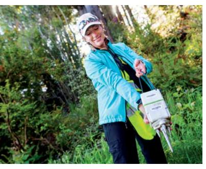
One of nearly 50 seismometers or nodes that Geology students like Kari Stockdale (ABOVE) installed in Arcata along fiber optic cables.
